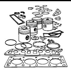
Inframe Overhaul Kits include: sleeves and orings (when required), pistons, rings, piston pins and retainers, rod and main bearings with thrusts, head gasket set, and oil pan gasket set.
