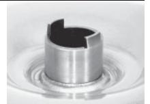
20 Size 11" Borg Warner Hub Removable Geared Hub W/8 Allen Head Bolts Pilot .787" OD Mounting 4 Square Mounting Nuts Stator Splines 19 Turbine Splines 15
