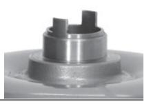
80 Size 13" Daikin Hub Geared Hub Pilot .982" OD x 1.10" L Mounting 6 Threaded Holes Stator Splines 27 **Turbine Splines 19**
