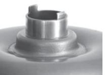
Comment: Fits early style F03 series pneumatic tire truck; 2 dowel pins at drive plate mounting.
