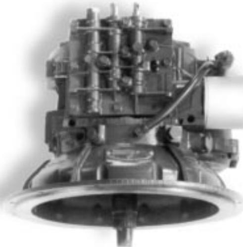
Top-down view of the PRL transmission with its manual valve assembly.
